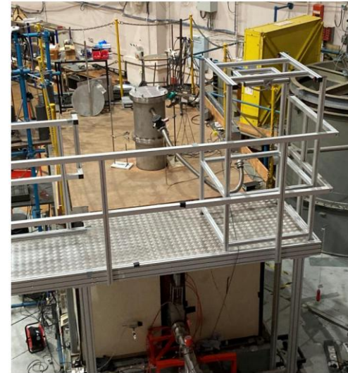
NPL thermal pile (6 m 3 of graphite)
