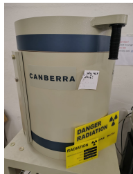
Figure 7: HPGe detector with Canberra electronics (left) and scheme of the detector with its main parameters (right).
